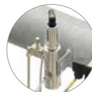
Outlet PDP sensor
